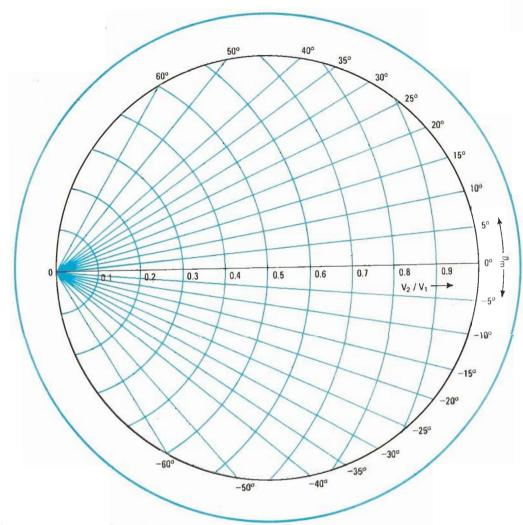
**2. Graphical solution.** The value of complex impedance Z, normalized with respect to noninductive resistor  $R_8$ , can be found graphically from this modified Smith chart. The chart establishes the coordinates for the voltage ratio of  $V_2/V_1$  and the relative phase shift of  $\theta_m$ .
