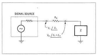
1. Test setup. Unknown complex impedance Z can be determined by measuring the voltage drop and phase shift across noninductive resistor  $R_s$ . Complex impedance Z can then be found graphically with a modified Smith chart or mathematically with a calculator.
